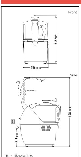
Electric Supply voltage: 380-440 V/3 ph/50/60 Hz Electrical power, max: 1 kW **Total Watts:** 1 kW Capacity: 2.5 kg/Cycle Performance (up to): **Capacity:** 5.5 litres Key Information: External dimensions, Width: 256 mm External dimensions, 415 mm Depth: External dimensions, Height: 482 mm
